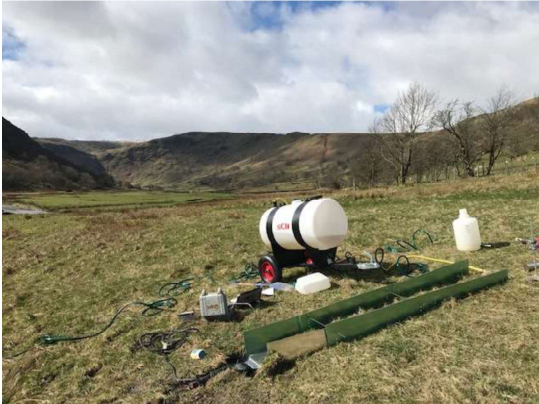
Above: Equipment being used by Stephanie Bond of Water@Leeds, as part of a PhD study to measure the rate of flow of water through different vegetation types [Photo: Stephanie Bond]
